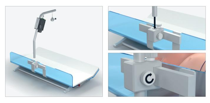
2. Pull out the black locking bolt and turn it 90°. The locking bolt stops in an open position.
