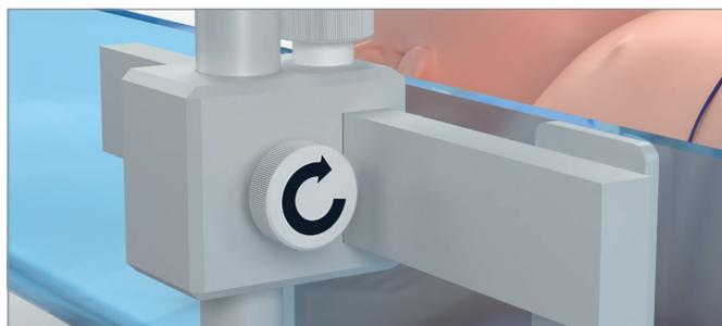
2. Pull out the black locking bolt and turn it 90°. The locking bolt stops in an open position.
